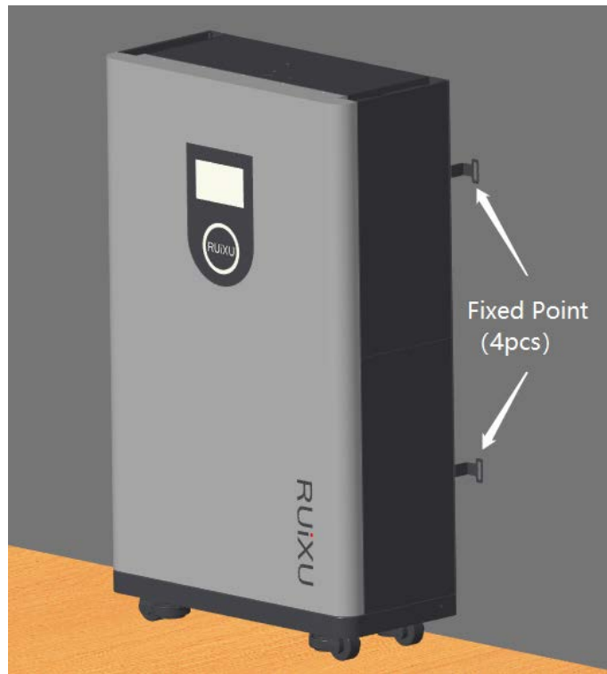
Battery fixation diagram (Installation torque: 9N)
